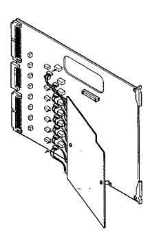
2. Place the Character board on the Camera Input board and plug in the boards.
