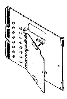
Fix both boards with the two supplied screws (M3x6) as shown below.
